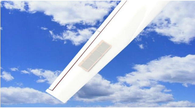
Figure 17 - Photography performed by SolidWorks program in a full scale representing the wing UAV with P-ESPAR antenna placed.
